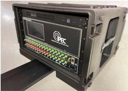
ASM-P is a Partial Discharge monitor for medium term testing of cables and switchgear. Based on the highly successful ASM system for permanent installation, the ASM-P is installed into a substation for 4 weeks or more in order to build up a picture of the condition of plant assets where high PD levels may have shown during a spot test and a temporary monitoring system needs to be implemented to ensure asset health in the short term.
